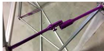
2. Insert the female arm into the frame hub.
