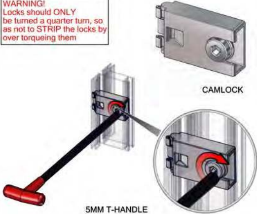
LOCK EXTRUSION BY USING 5MM HEX KEY
