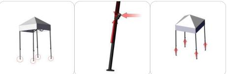
The frame will have four slide locks, one for each corner. When the tent scissor frame is fully extended; make sure the prong of the slide lock snaps into the tube locator hole. Press the lever on the slide lock to disengage the prong from the tube allowing to slide the lock up or down during assembly.
