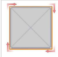
Your opaque liner will attach to the top of your tower with hook and loop fastener on the liner and on the top of the extrusion.
