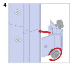
Using the screws provided, attach 8 of the brackets to the joints of your verticals and two at the top of you PMFC2 verticals.
