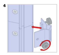
Using the screws provided, attach 8 of the brackets to the joints of your verticals and two at the top of you PMFC2 verticals.
