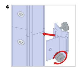
Using the screws provided, attach 8 of the brackets to the joints of your verticals and two at the top of you PMFC2 verticals.
