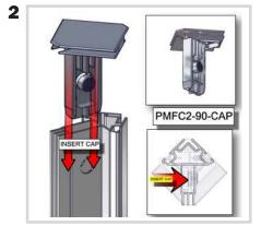
Push down on the snap button on your cap and push it into the top and bottom of the vertical posts until it snaps in place.
