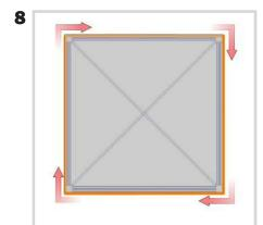
Your opaque liner will attach to the top of your tower with hook and loop fastener on the liner and on the top of the extrusion.
